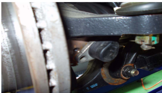
Fig. 5. Example of a loose bolt to fix wheel speed sensor.
