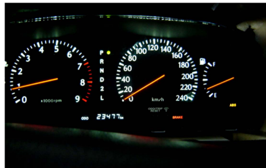
Fig. 8. ABS warning lamp example of instrument panel.
