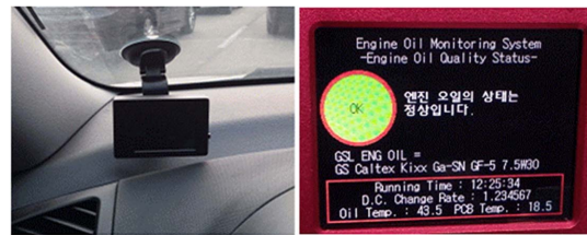
Fig. 7. Individual display device and a sample screen frame.
