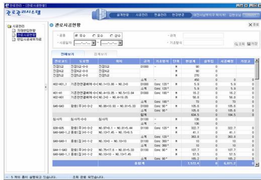
FIGURE 6 PIPELINE CONSTRUCTION MANAGEMENT SYSTEM
