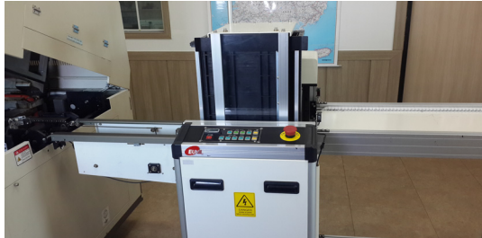
[Fig. 7] SMT equipment for producing a test product of multi-channel LED light driver
