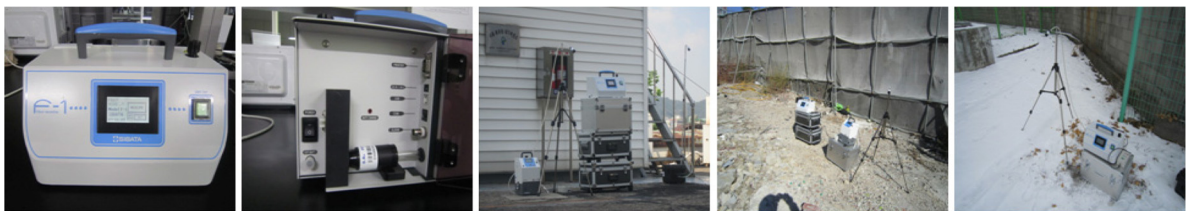
Figure 2. Sampling view for the airborne asbestos with KF-100 and PCM
