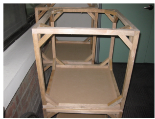
Photo 5 Box of thermal insulation performance mock-up test
