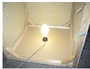
Photo 6 Heat source of thermal insulation performance mock-up test
