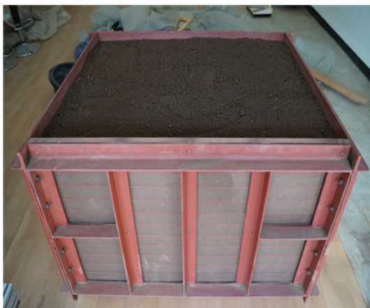
Fig. 2. Soil box for small-scaled lab. test.
