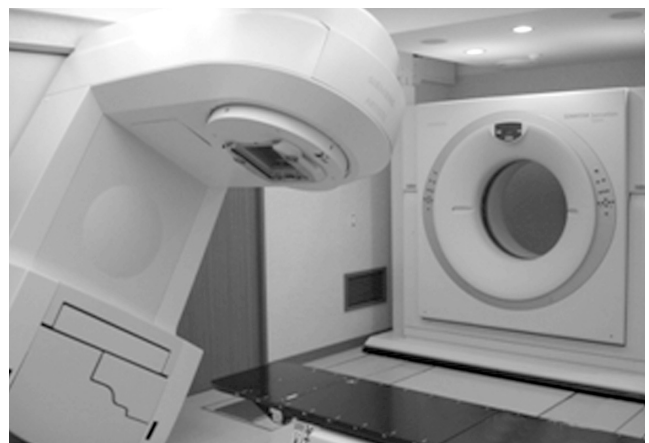
Fig 1. The image of CT on rail. It consist of LINAC(ARTISTE, SIEMENSE) and CT scanner (Sensation open , SIEMENSE)
