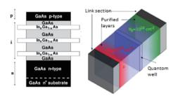
Fig. 6. A solar cell p-i-n quantum well structure
