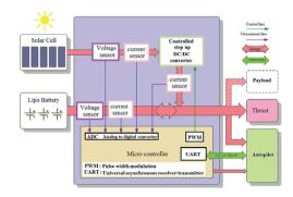
Fig. 4. Diagram used for the usage of hybrid energy in fixed wing
