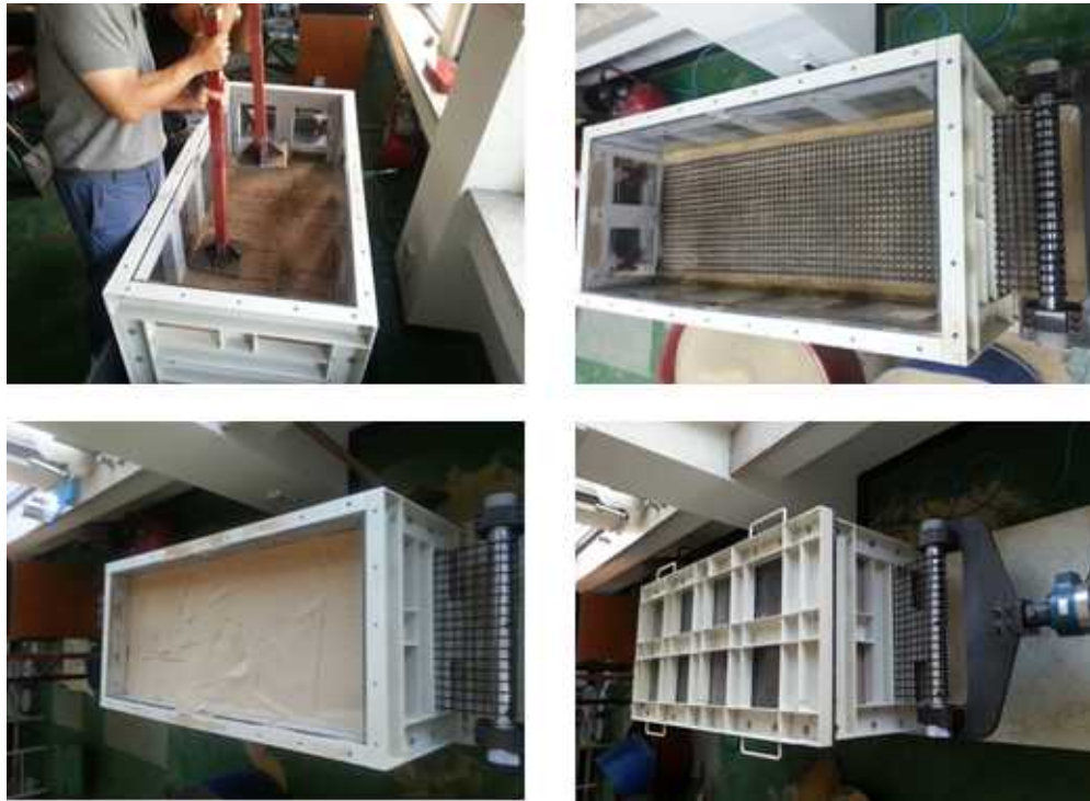
Fig. 2 The pullout device and test preparation
