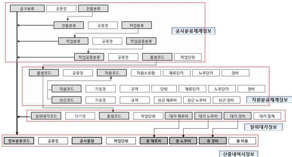
Fig 5. Relational Data Base Structure for Automated Cost Estimating
