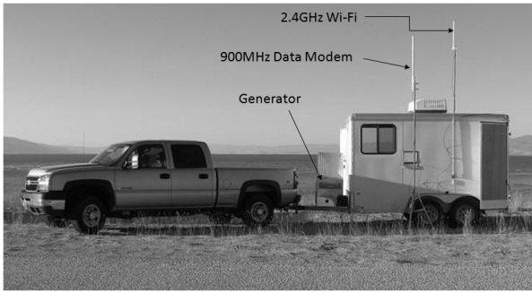
Fig. 8. Ground Control Center
