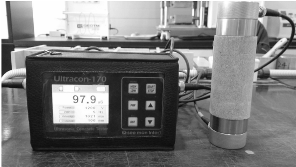
Fig. 4. Test Set-up for Determination of Pulse-travel Time
