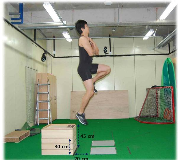
Figure 1. Landing heights & force plate condition
