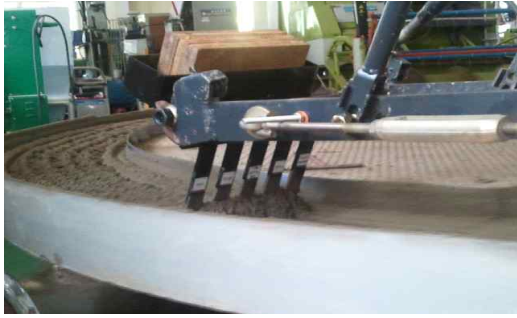
Fig. 2. Anti-abrasion material selecting test in soil chamber.
