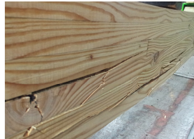
Fig. 4. Failure shape of the glulam after bending test (Larch).
