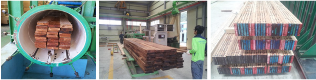
Fig. 1. The process of fire retardants treated Glulam.
