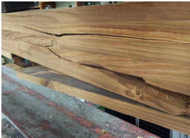
Fig. 3. Failure shape of the glulam after bending test (Korean pine).
