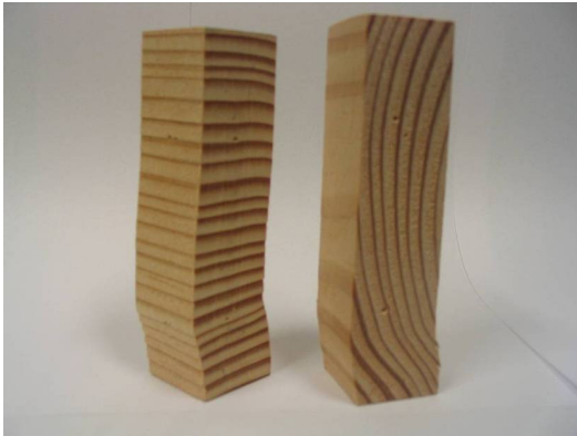
Fig. 9. Actual deformed shapes of the radial and tangential specimen overloaded.
