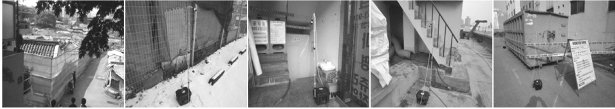
Fig. 3. Field sampling view for analysis of the airborne asbestos concentrations.
