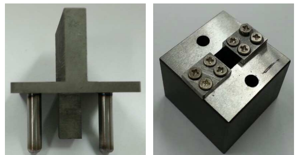
Fig. 1 Punch (left) and die (right) used in experiment
