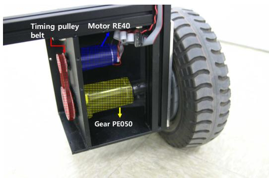
Fig. 5 Powered wheel part
