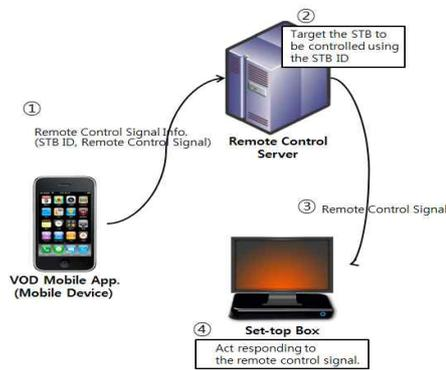
(Figure 8) Process of Handling Remote Control Signals
