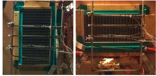
Horizontal position Vertical position Fig. 6 Photo of performance experiment as a position of thermoelectric generator at calorimeter.
