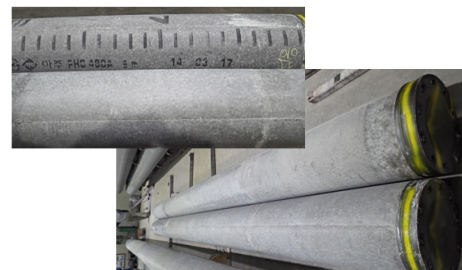
1st steam curing
