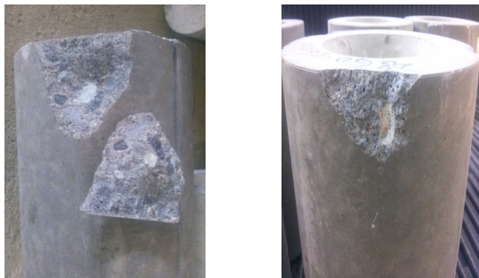
Fig. 5. Pop-out after 2nd High Temperature and High Pressure Curing
