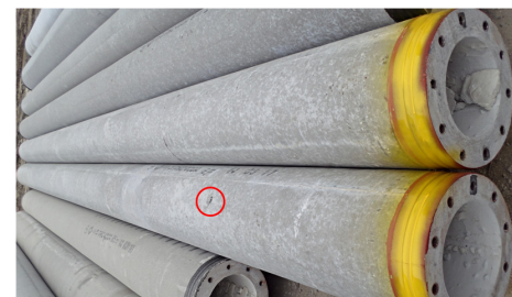
2nd high temperature and high pressure curing
