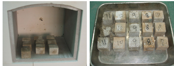
Fig. 11. Specimens after fire-resistance test
