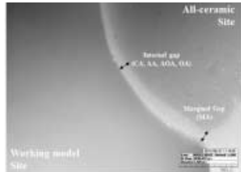
Fig. 4. Measurement of margin and internal gap using digital microscope at 160x magnification
