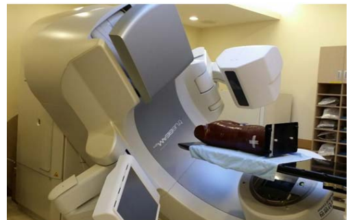
Figure 2. Set-up of Rando phantom to measure photon neutron dose on TrueBeam Stx
