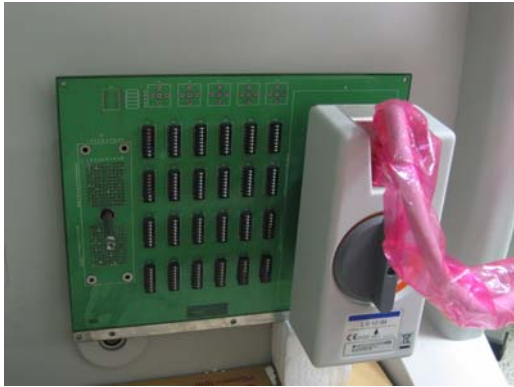
Figure 2. An experimental panel for electrically disconnecting the piezoelectric elements of the ultrasonic probe.
