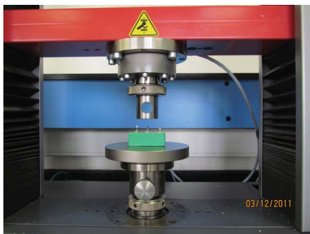
Fig. 1. Root fracture is induced using an Instron testing machine.
