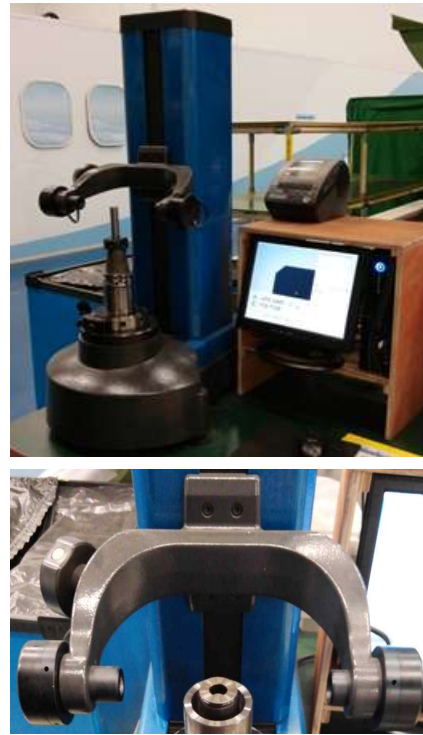
<Fig. 9> Installed tool presetter and vision module
