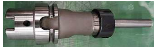
<Fig. 14> Standard initial alignment device
