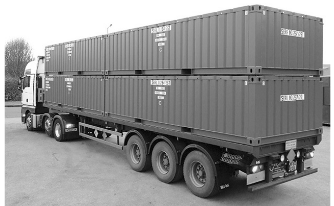
Fig. 3. Half-height Disposal Containers.
