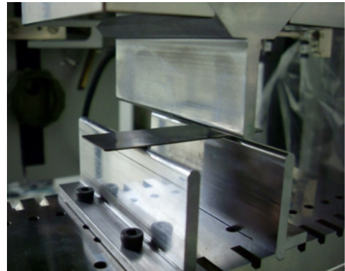
[Fig. 2] Jig of bending test
