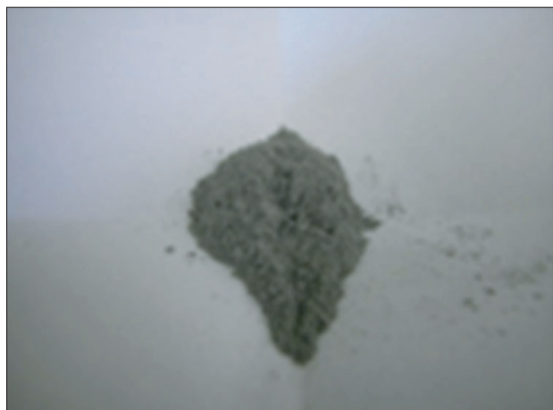
Fig. 4. Optical image of AlN powder synthesized under the condition of Al-10 wt.% Mg-N.
