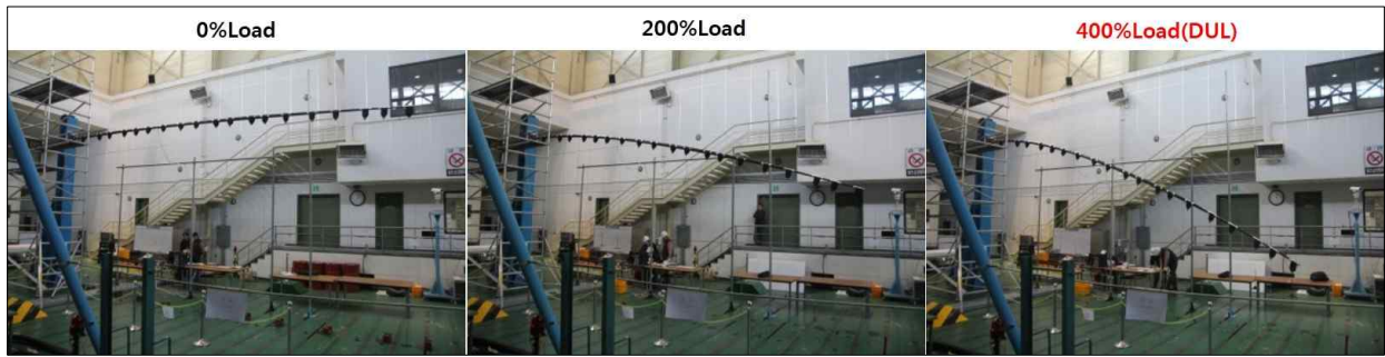
Fig. 8 Static Test for Spar Design B
