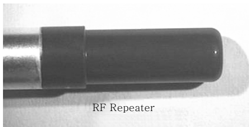
Fig. 5 RF repeater coated by PEO process
