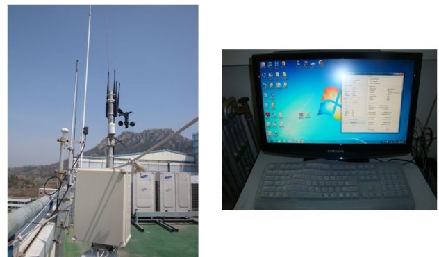
Fig. 8. AIS receivers to collect traffic data within Mokpo VTS area (left) and SQL Server to compile the data (right).
