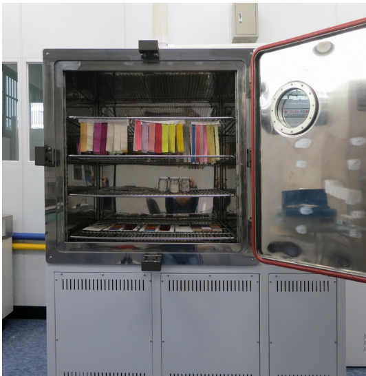
Figure 1. Effect test on materials in anoxic chamber system.
