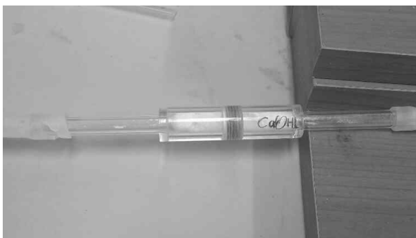
[Figure 3.5] Catalyst reactor
