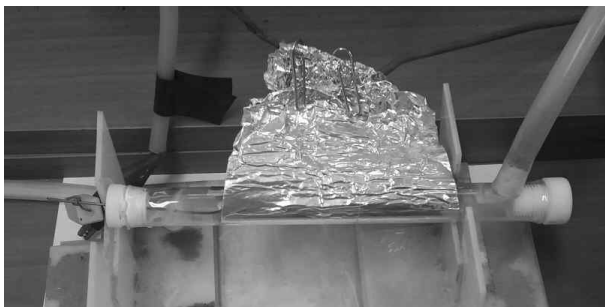
[Figure 3.4] SPCP reactor
