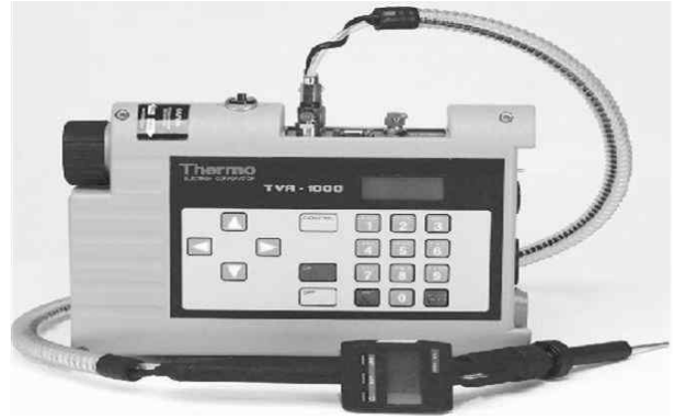
[Figure 6] Total hydrocarbon measurement equipment(TVA-1000B,Thermo Environmental Instrument, U.S.A)
