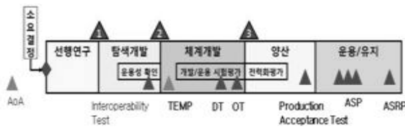
[Figure 1] T&E and live fire test in the full life cycle of weapon systems development.
