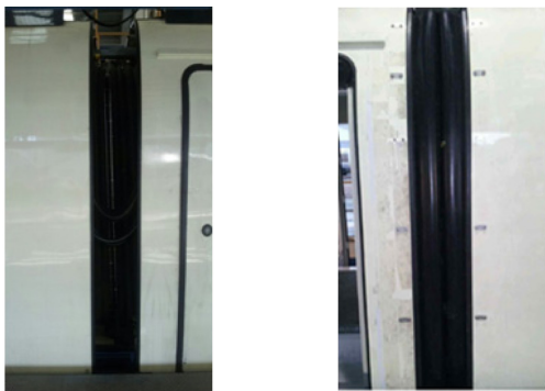
(a) Installation of side fairing : before (left) and after (right)
