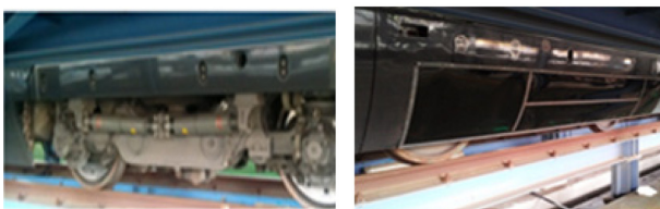
(b) Installation of bogie cover : before (left) and after (right)
