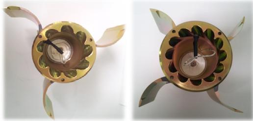
Fig. 6 Configuration of the 3 tailfins-9 flutes(left) shaped and 4 tailfins-12 flutes(right) shaped nozzle assembly.
