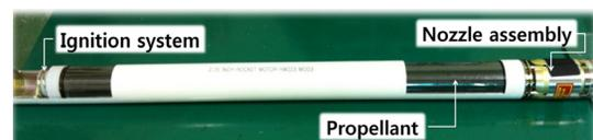
Fig. 2 Korean 2.75 inch rocket propulsion system.
