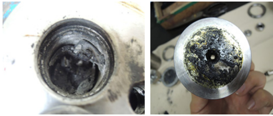
Fig. 9 Igniter storeroom(L) and nozzle(R) after the combustion test with 4 g of MTV.
