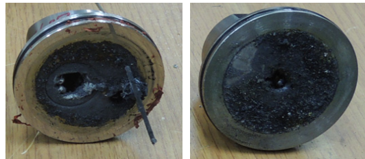
Fig. 10 Igniter storeroom exit(L) and nozzle(R) after the combustion test with 6 g of MTV.
