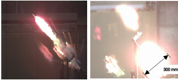
(a) ignited from aft (b) ignited from front/aft Fig. 5. Ignition pattern of flare after discharging
