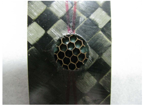
Fig. 9. Insertion of honeycomb core plug in removed area
