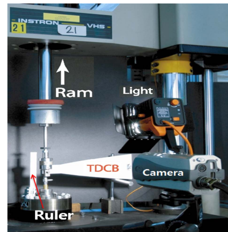
Fig. 3. Setup of aluminum alloy at impact tester
