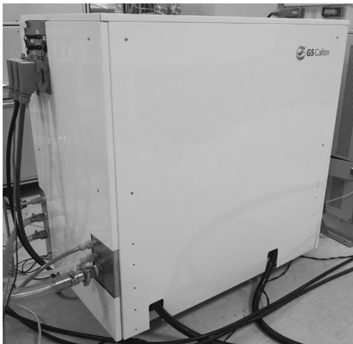
Fig. 6 Photo of the 25kW-class PEM fuel cell system
