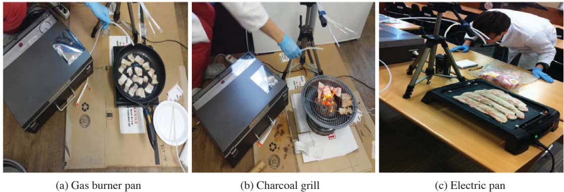
Fig. 1. Illustration of gas sampling system from cooking of pork belly meat.
