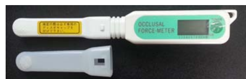
Fig. 1. Hydraulic pressure occlusal force gauge
