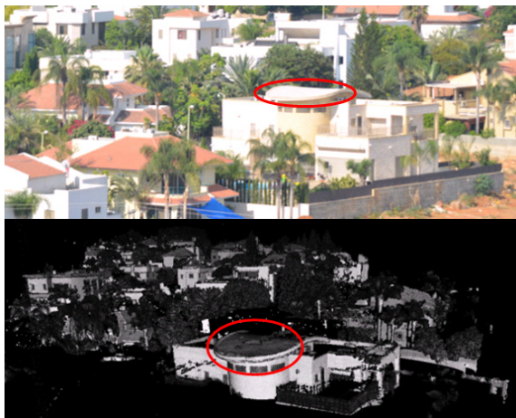
Fig. 4. The 3D Image of the Test Site by the Laser Radar
