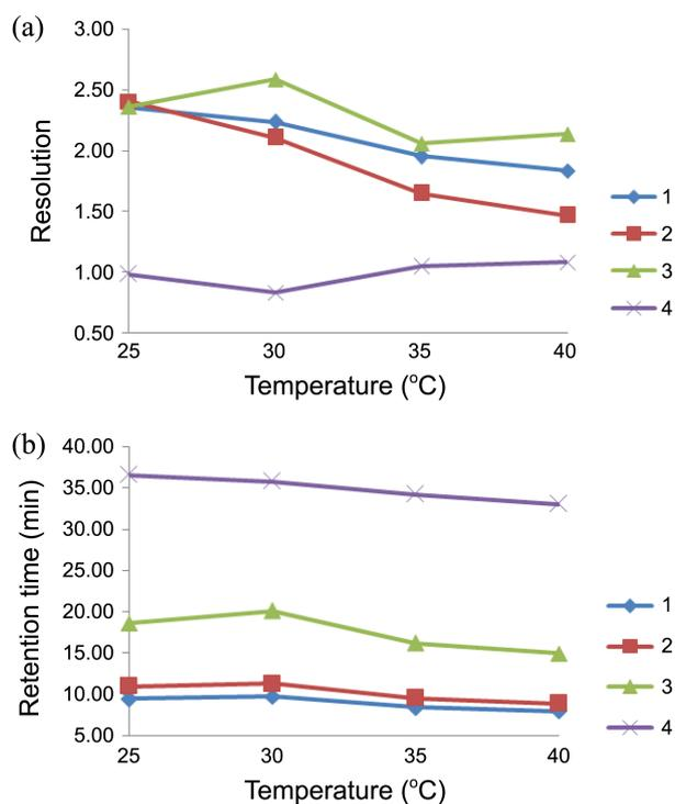
**Figure 5.** Effect of separation temperature on the retention time of four marker compounds (a) and on the resolution of the adjacent peaks (b).
